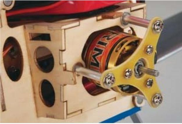
The prebuilt motor box streamlines motor installation. It's light, strong and a perfect fit for the recommended RimFire™ 400 brushless outrunner.
