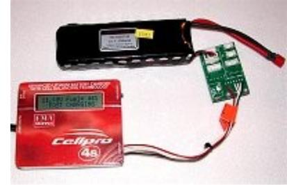
The best possible capacity retention for Li-Pos is obtained when you store them about half-charged and keep them cold around 0° (C) or 32° (F). This results in approximately 2% loss of capacity per year. The next best is a 4% loss per year when stored half-charged at 25° (C) or 75° (F).
