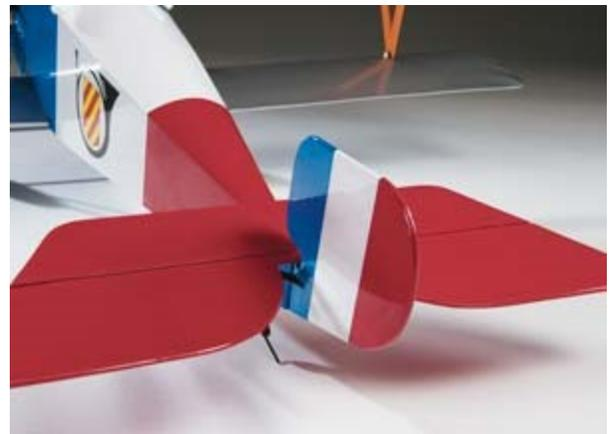
Both aileron and elevator control surfaces are pre-hinged to slash assembly time.
