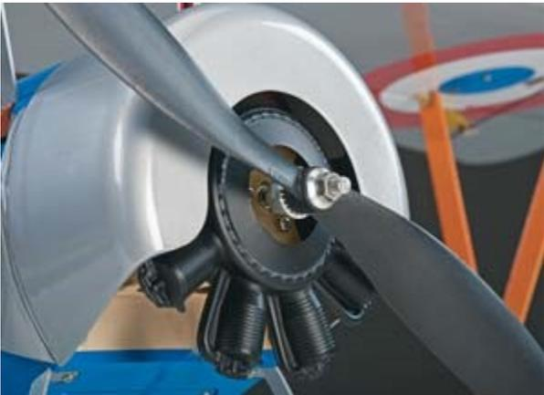
The replica rotary engine hides the motor, requires only the time it takes to drive two screws. The cowl requires even less; magnets align it and hold it securely, yet release quickly and easily for pack changes.
