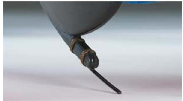
The tail skid appears to be lashed in place with rope, just as it was on the original. And there's no vertical fin; the entire surface pivots for powerful rudder response.
