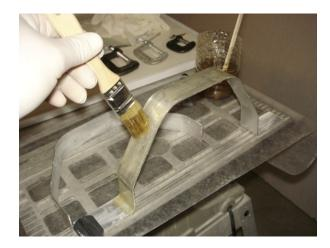
Tip: When applying resin, don't use brush strokes. This will distort the fiberglass and make it hard to do a good layup. Instead, dab the brush with short, quick motions.
