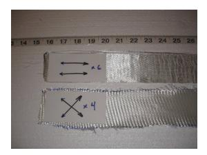
All your fiberglass strips should be 1 inch minimum longer than the gear. They should be wider than your finished gear by at least 1 inch. This will make placement a lot less critical. When the resin has cured, you will cut the excess away.
