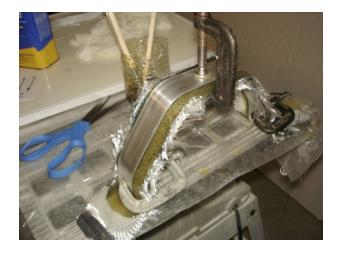
Put the top form on the layup and very lightly clamp it to the bottom form. Stop clamping when you squeeze just a little resin out. Make sure that all the clamps have about the same pressure and that the top and bottom forms align. You don't want to squeeze all the resin out! Caution: When using power tools, always use safety goggles and other protective equipment!
