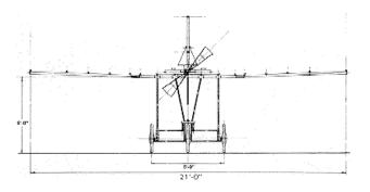
Whether or not Pearse flew in any acceptable sense, and regardless of the exact date, his first aircraft was a remarkable invention embodying several farsighted concepts: a monoplane configuration, wing flaps and rear elevator, tricycle undercarriage with steerable nose wheel, and a propeller with variablepitch blades driven by a unique double-acting horizontally opposed petrol engine.
