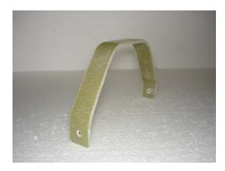
Next, drill holes for the axles. You can use bolts from the hardware store or the hobby-shop variety. Be sure to use a lock washer or lock nut for the fist nut if you are not using hobby shop axles. Last, drill the holes to attach the gear to the airplane. I have used 1/4-20 nylon bolts for this task. The nylon bolts shear in a crash, but hold up well in hard landings.
