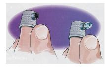
fingertip and the metal hardware item on the magnet. Now guide the item to that hard-to-reach spot and install it. Thimbles come in several sizes, and the new mini magnets are very strong and will hold nuts, screws and other metals securely. This is also ideal for retrieving small screws and nuts that fall deep into the model.
